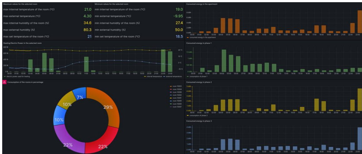
Figure 24: An example of a prototype Grafana dashboard which is connected to the new periodic measurements database in Timescale II
