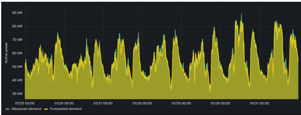
Figure 32: Measured vs. forecasted demand of the community battery installation in Crevillent.
