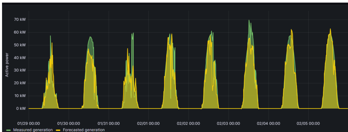
Figure 33: Measured vs. forecasted generation of the community battery installation in Crevillent.
