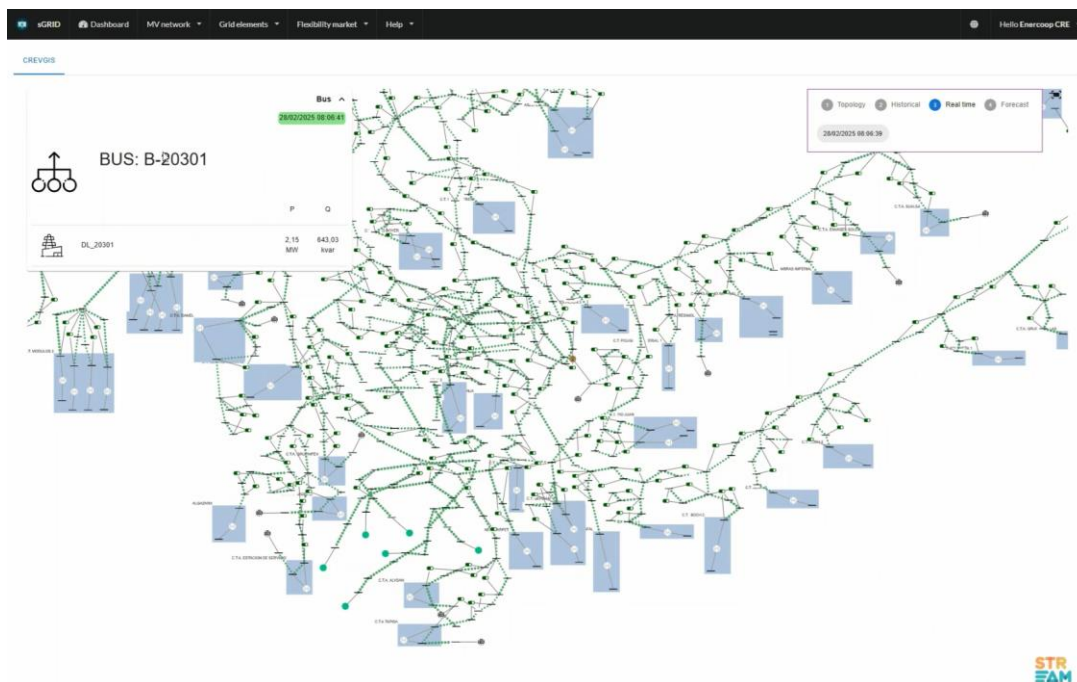
Figure 46: sGRID (ES) Dynamic representation of power flow calculation in Crevillent MV grid.
