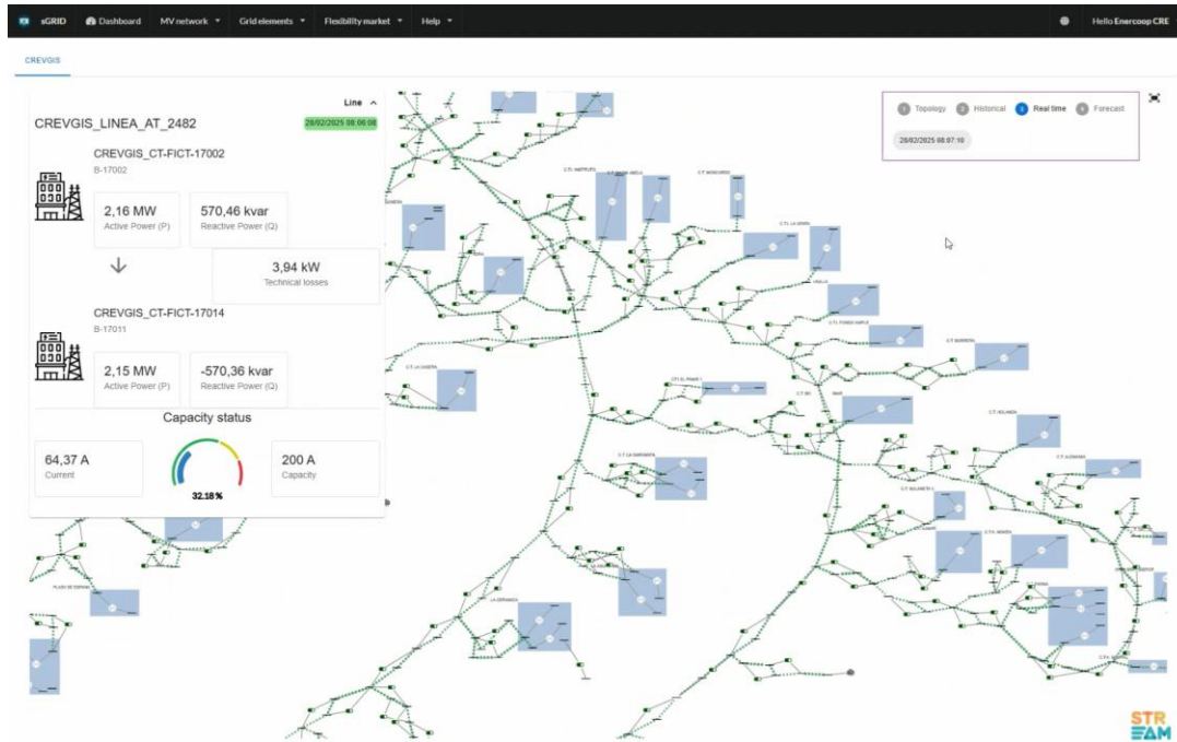
Figure 47: sGRID (ES) Power flow results of a specific MV line in Crevillent.
