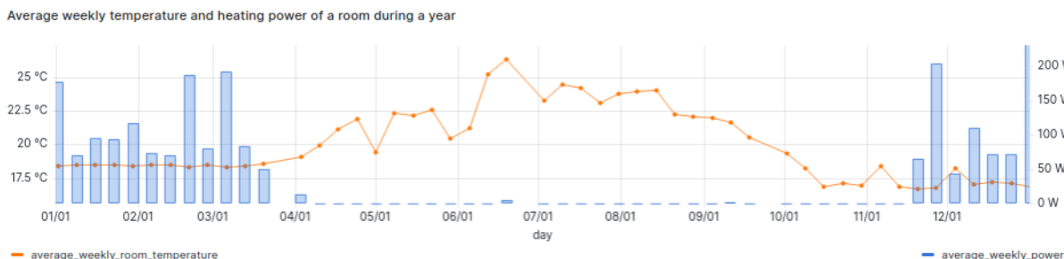
Figure 79: Average weekly temperature of a room and average weekly power used for heating that room.
